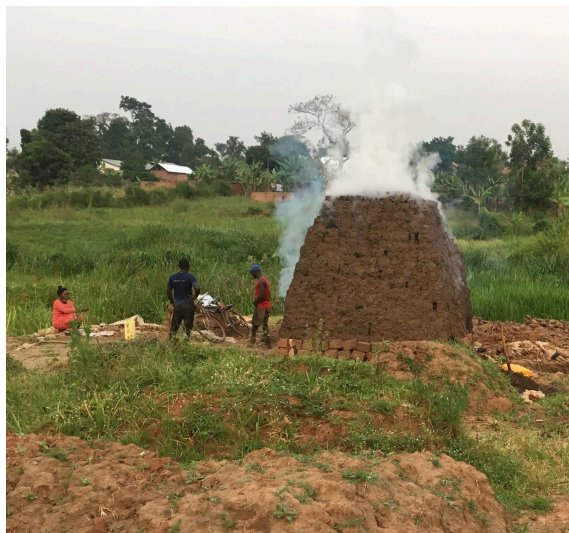
Clay being harvested near Kamuli, Uganda, is being made into bricks in this oven on site. Photo credit: Amber Anderson.
